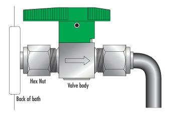
Figure 1 Drain Valve Installation—IMPORTANT: Do Not Over Tighten. Follow the installation instructions above.
